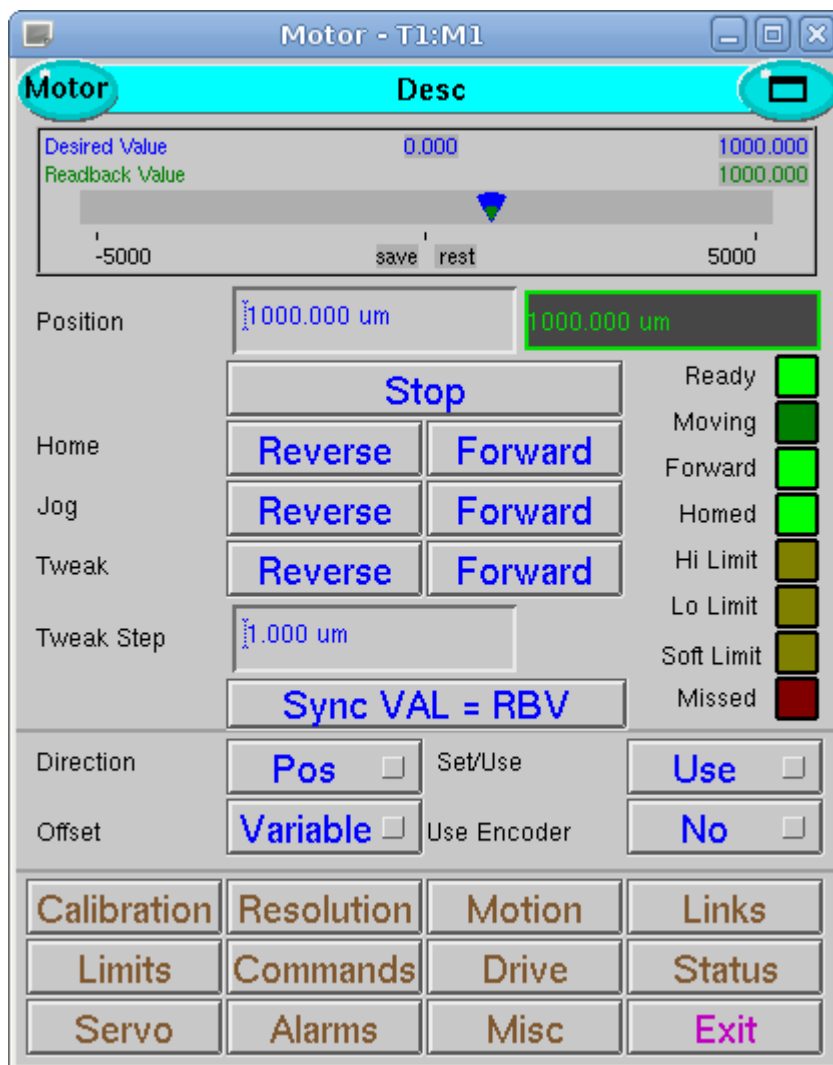
Figure 3 Motor axis control screen.
