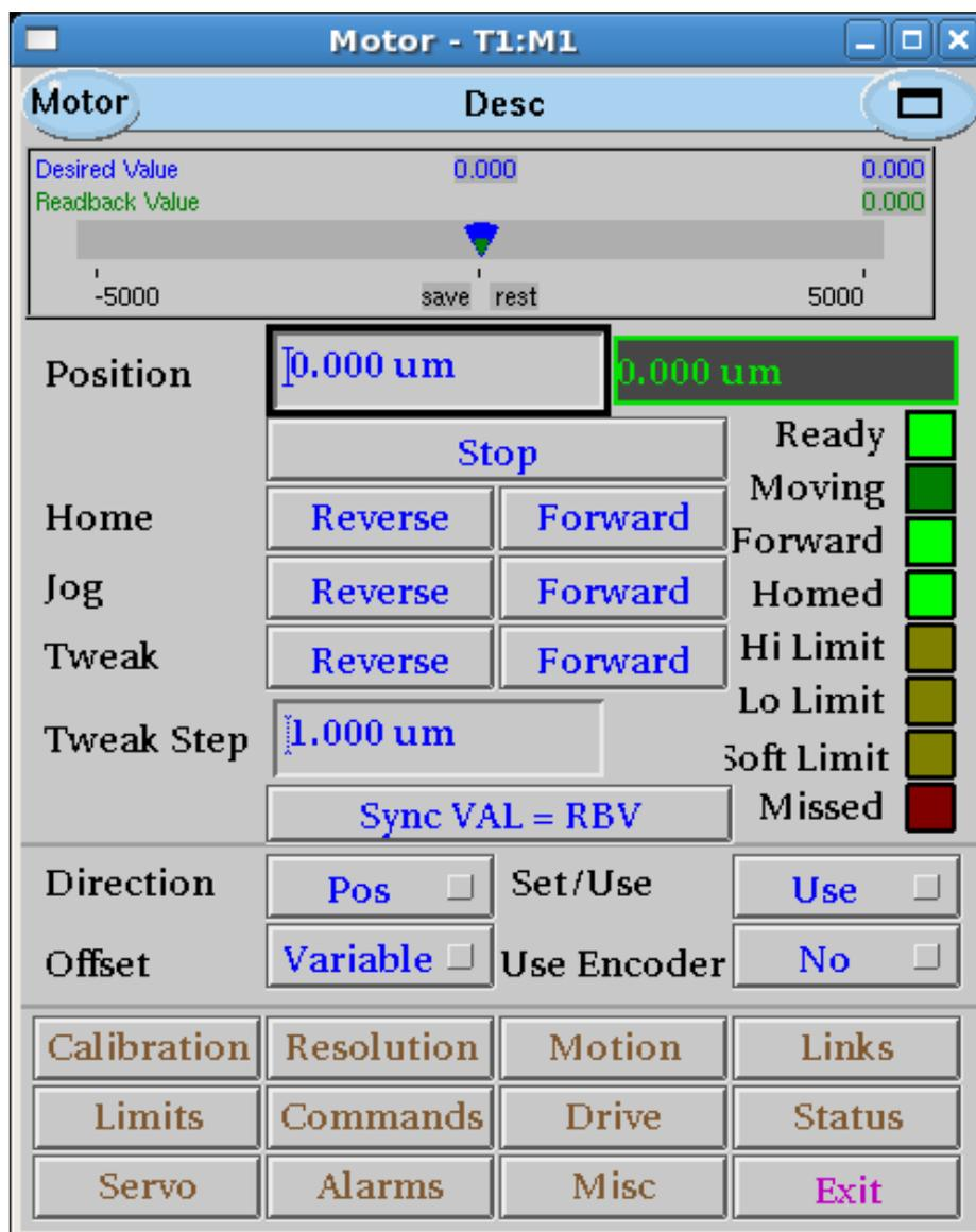
Figure 8 Motor record control screen example.
