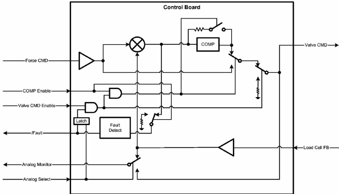
Figure 7, Analogue Force Control Loop
