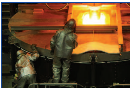
(Above) Casting the ATST primary mirror: photo courtesy SCHOTT AG. (Top right) Artist's impression of the ATST; picture courtesy of NSO/AURA/NSF
